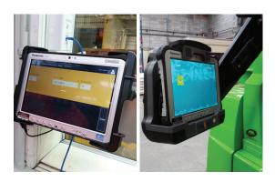
O'Donnell says placing the 26 Toughpads in the factory was achieved with fully rugged Havis mounts for those in fixed locations; for those mounted on forklifts, some further ingenuity was required. "Together with a local engineering firm, we developed a special arm to hold the devices. A lot went into that, to make sure the Toughpad is ergonomically positioned, while still allowing the operator to 'bail out' should it be necessary," he explains.
