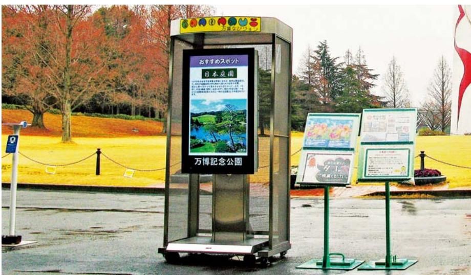
Banpaku Navision uses durable LCD displays fit for outdoor applications. DIGITAL LINK is used to connect the outdoor displays to the image source equipment set up indoors.
