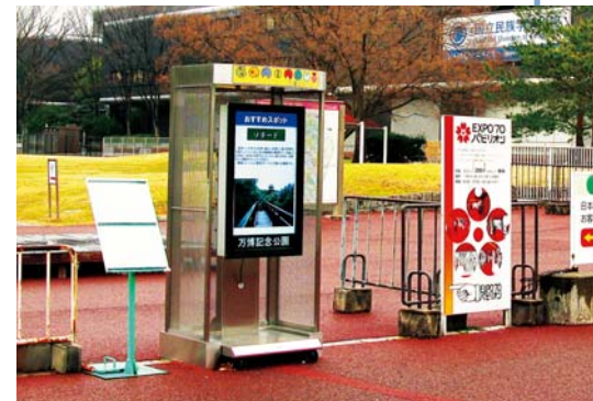
The housing is designed to cover the entire display unit to prevent injury by bumping into the display corners.
