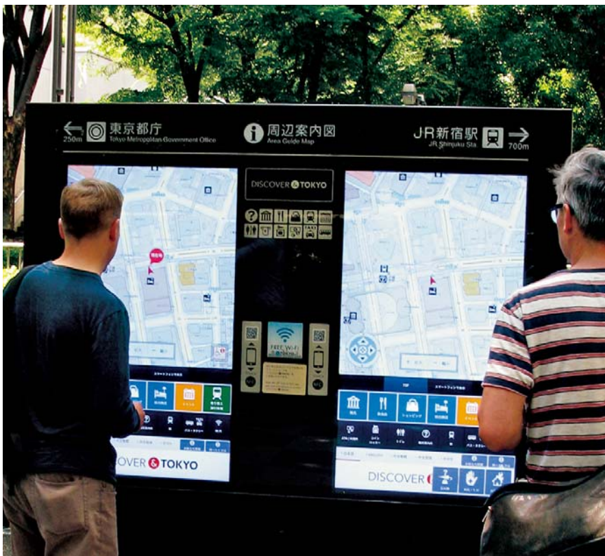
The high-performance tourist guidance signs attract the attention of people walking by them with their with vivid images. By providing icons that let the viewer switch the content at the bottom of the screen, the displays are also handicap-accessible.
