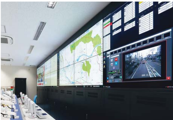
▲ An IPS LCD panel, with excellent color reproduction and a wide angle of view, is used. The image can be clearly seen all the way from the command table at the end of the room.
