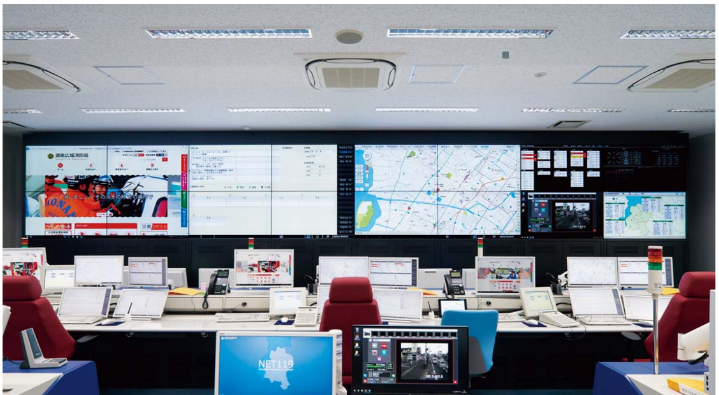
The ultra-narrow bezel design displays all of the necessary information in an easy-to-see manner. The large multi-screen system has two TH-55LFV6 displays mounted vertically and eight TH-55LFV6 displays mounted horizontally.
