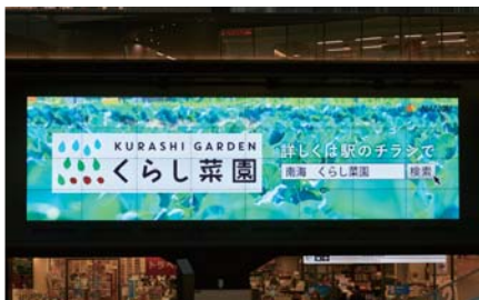
▲ Considering the load-bearing capacity and viewing angle, the wide-screen system comprises 32 displays (4 vertical x 8 horizontal).
