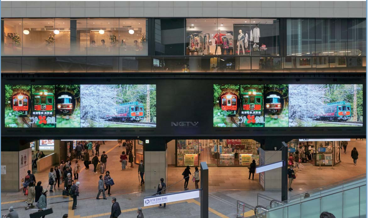
▲ Namba Galleria Twin Vision features 32 LCD 55-inch display screens aligned in two units.
