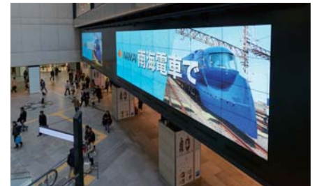
▲ The IPS LCD panel was used to prevent brightness and color changes when viewed from almost either side.
