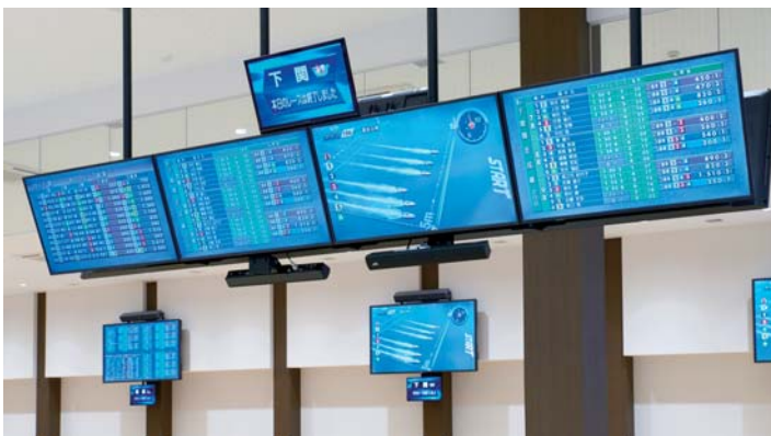
▲ Ceiling suspended TH-43LFE8 displays are installed in the middle of the venue. Four displays serve as a set to display information from a single venue. Eight sets are installed within the venue, covering races from eight different venues.
