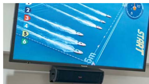
▲ A WS-LA50 array speaker is installed for each display.
