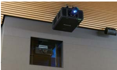
▲ The PT-RQ13K (top) projects the main images, while the PT-RZ970L (bottom) displays an abridged version and event information.
