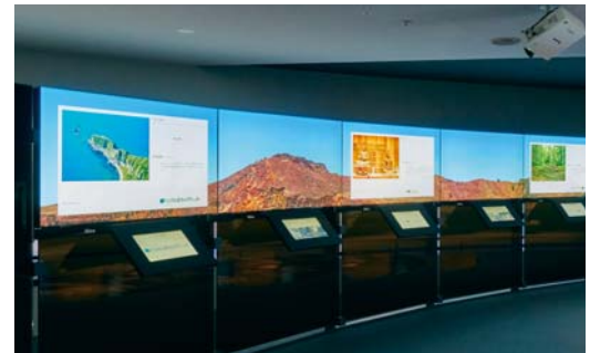
◀ The multi-screen display consisting of nine displays arranged in a row horizontally at the “Holy Mountain” exhibition zone. By selecting the content that you wish to learn about on the touch panel installed underneath the displays, a pop-up commentary is displayed on the display above.
