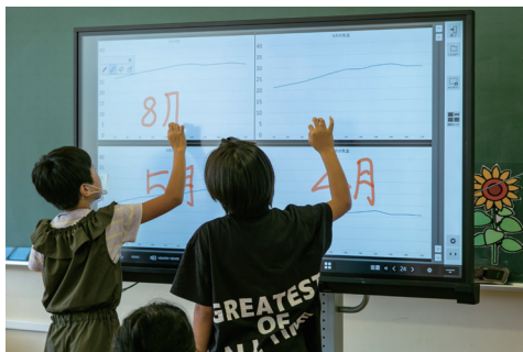
▲Using the multi-screen comparison feature to show spring-summer temperature graphs on four panels. You can write on the screen with your fingers, and when using Windows the screen can be touched at up to 20 points at a time.
