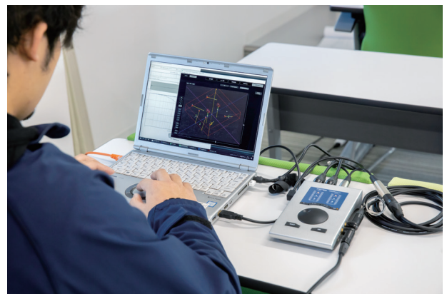
▲ Based on results measured by the microphone, it automatically calculates FIR coefficients to get close to the target characteristics without disrupting the phase.
