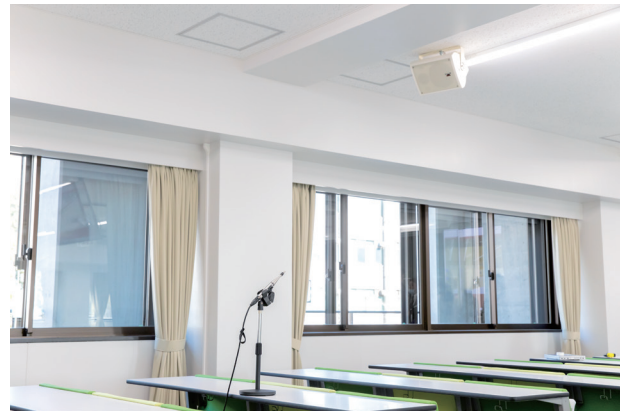
▲ The acoustic simulation using PASD. A measurement microphone pointed at the speaker collects test signals.
