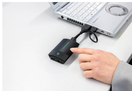
▲ You just need to press the main button to start screen-sharing. Just press the sub button on the end to change to multi-screen, which shows up to four screens.
