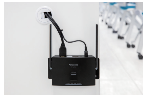
▲ The PressIT receiver located at the edge of the podium. One receiver can connect to up to 32 transmitters.
