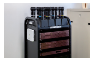
▲ In Seishinkan, which was renovated in 2020, WX-SR200A Series receivers, antennas and 16 microphones are stored in a portable rack. It is DECT-compliant, so it can also be moved to be used in another classroom.
