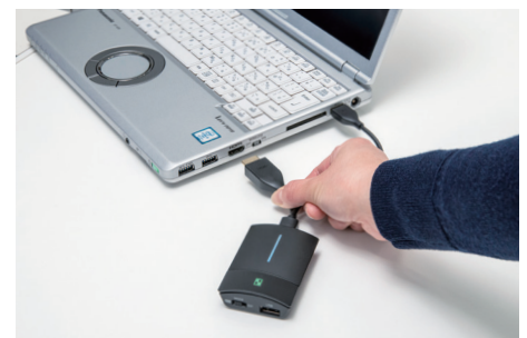
▲ The device is extremely easy to use—just plug it into the PC's HDMI port. The USB connector is for charging.
