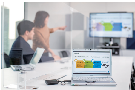
▲ PressIT connected to a PC. Screen-sharing is now possible even from locations where cables cannot reach.
