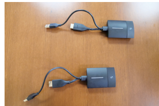
▲ PressIT transmitters. Two transmitters are used in discussion-type meetings.
