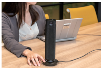
▲ The screen splitting mode can be changed simply by pressing a button on the unit. There are also buttons to turn microphones on and off and adjust the volume.
