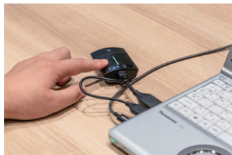
▲ The Wireless Presentation System "PressIT": simply plug the transmitter into a computer and press the button to share the screen in another screen or display
