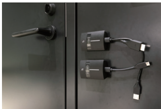
▲ The PressIT attaches to the door of the conference room with a magnet and can be used straight away (top: HDMI™ connection, bottom: USB Type-C connection)
