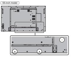
• The positions of the holes are the same for 42-inch and 49-inch models.
