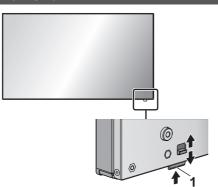
To take out/store the power indicator and remote control sensor, operate the lever on the rear panel.
