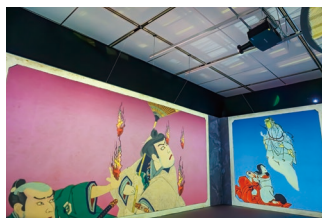
▲ The front wall of Yokai Gathering used a PT-MZ20K projector paired with the ET-EMU100 ultra-short-throw lens for vivid, close-range projection.
