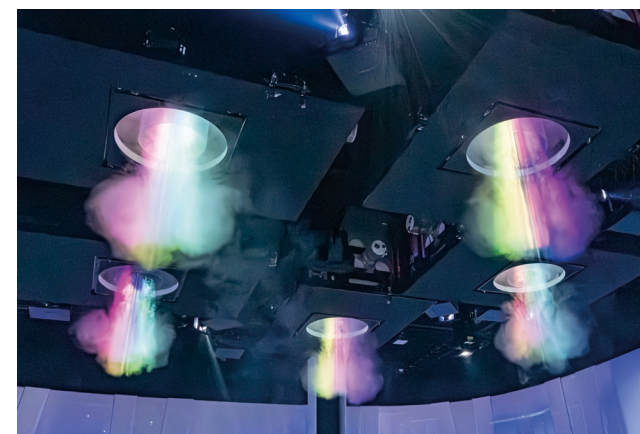
▲ Vortex rings projected clear imagery onto the floor from a 5-meter-high ceiling
