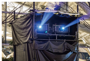
▲ PT-RQ25K units projecting the main visuals (two units on each side at the rear of the venue).
