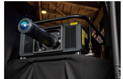
▲ The system included a PT-RQ22K 3-Chip DLP® Laser Projector equipped with an ET-D3LEF70 Fisheye Lens. The projector was placed on a platform to prevent participants' shadows from appearing on the screen
