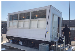
▲ Trailer housing five PT-RQ50K projectors with precise temperature control
