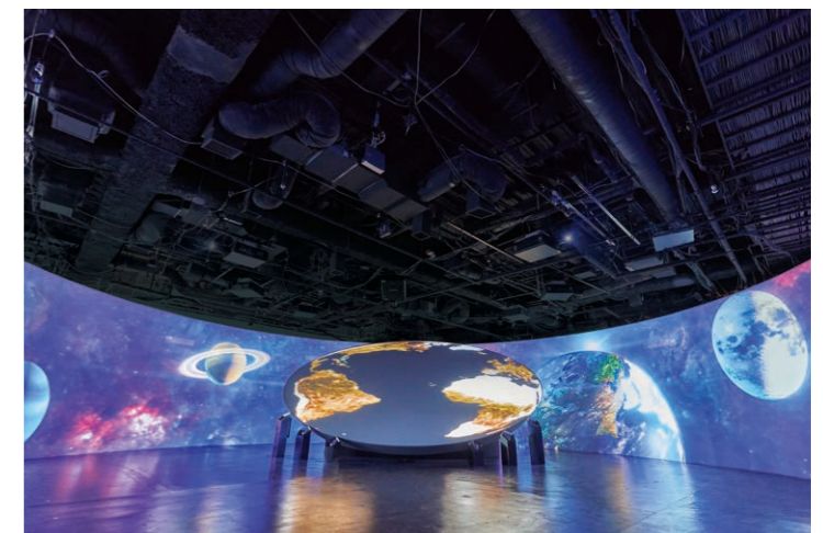
▲On the final leg of the journey, a vast panorama is created by using six PT-RZ870JL 1-Chip DLP® Laser Projectors: the use of multiple units allows for seamless merging of the images together, and what's more, in the center of the room is a large disk that uses PT-RC010JL 1-Chip DLP® Laser Projectors to project an image of Mother Earth
