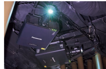
▲By combining the ET-DLE020 Ultra-Short-Throw Lens with the power of projectors in the DLP® lineup to convey images, clear, attractive projection is possible even on curved screens and narrow areas between the "trees"
