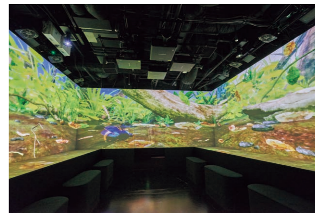
▲The Ant View Zone is meant to allow visitors to see the world of bugs and insects through the eyes of an ant, so three PT-RZ870JL 1-Chip DLP® Laser Projectors with ET-DLE020 Zoom Lenses (Ultra-Short-Throw Lenses) facing in three directions and two more facing the floor are used to create an immersive experience surrounded by the world of bugs and insects
