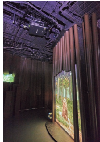
▲The ET-DLE035 is a Fixed-Focus Lens with a built-in mirror (an Ultra-Short-Throw Lens), so it can reflect images to the opposite side of the projector direction, significantly shortening the projection distance
