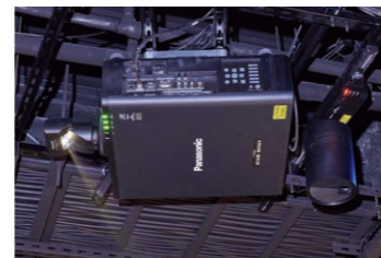
▲The ET-DLE035 is a Fixed-Focus Lens with a built-in mirror (an Ultra-Short-Throw Lens), so it can reflect images to the opposite side of the projector direction, significantly shortening the projection distance
