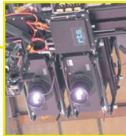
A stack of two PT-DS20K projectors allowed the badminton venue to be captured with 40,000 lumens of brightness. The rectangular image was used to cover the court size.
