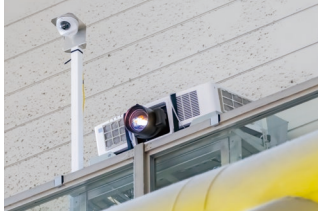
▲ PT-MZ20K projector and network camera for real-time projection monitoring
