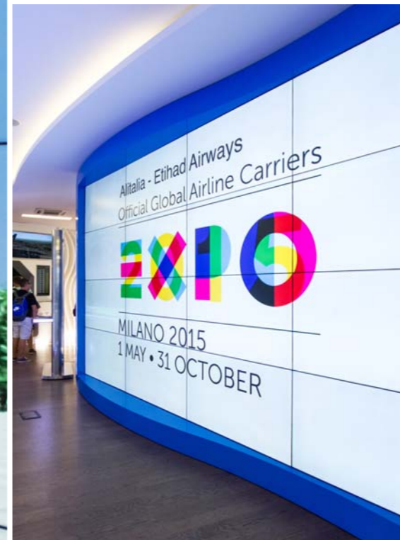
High-brightness panels with anti-glare/anti-reflection treatment assured maximum visibility even under strong artificial light.
