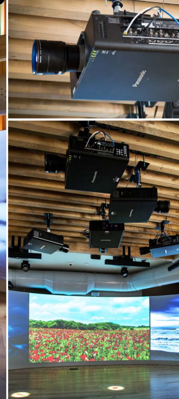
Seven 1-Chip DLP™ PT-DZ770Ks were used for floor projection.
